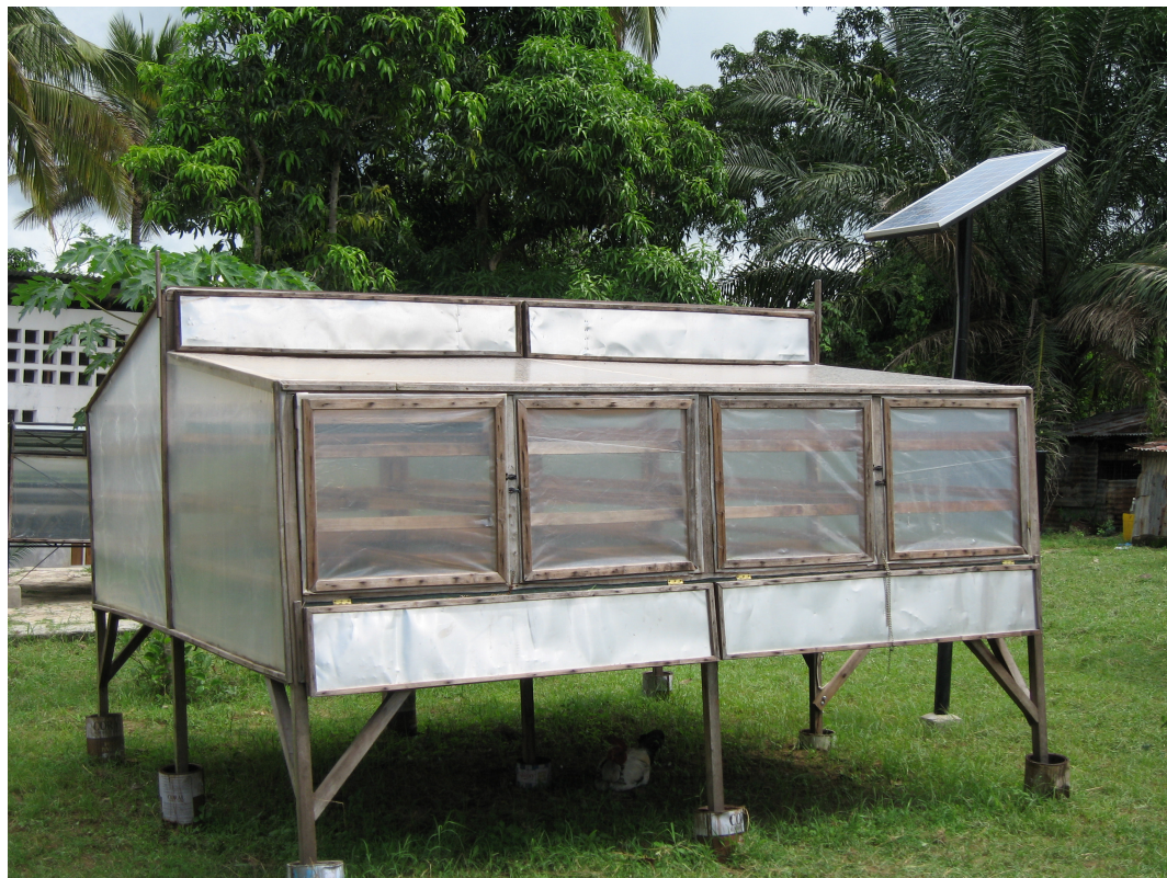
Figure 2.3: Modified cabinet solar dryer fitted with solar driven circulation fans
