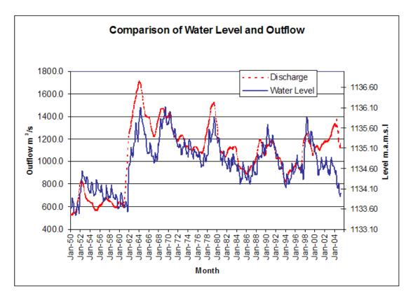
Figure 2: Hydrograph showing comparison of Nile outflow and Lake level, 1950-2005.
