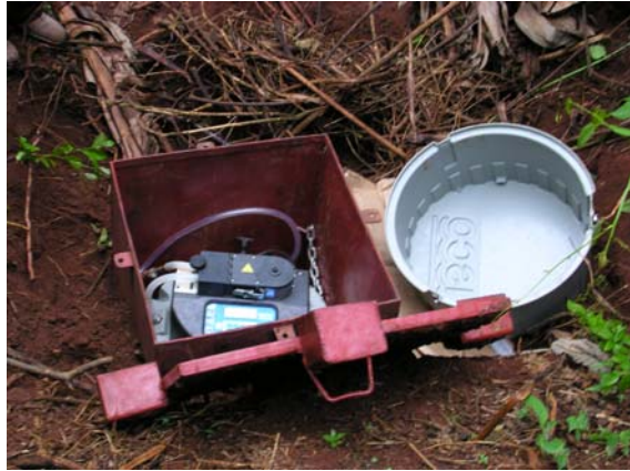
Figure 5.16: ISCO Autosampler Installation at the Dionosoyiet Wetland Transect
